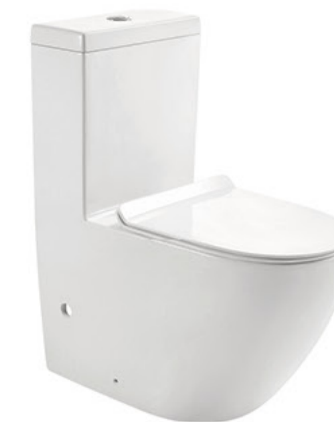
8221 Washdown/Siphonic One-piece Toilet Size: 700x370x855mm P-trap: 180mm Roughing-in S-trap: 250/300mm Roughing-in
