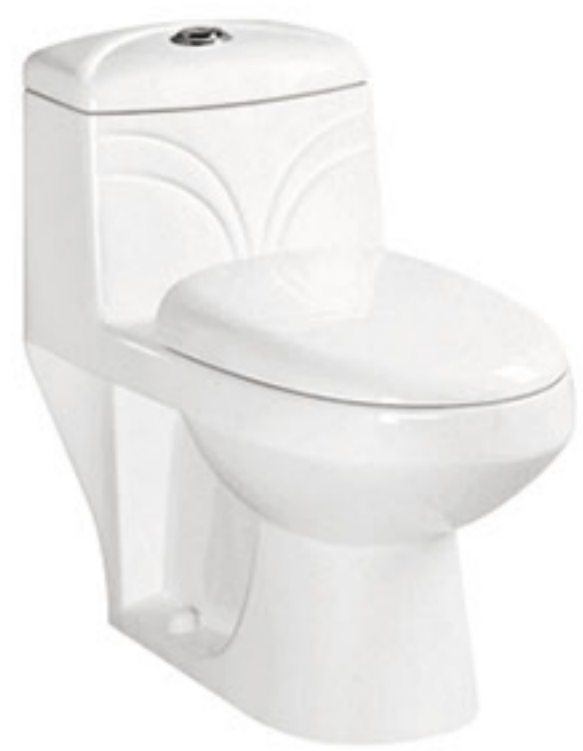
8245 Washdown One-piece Toilet Size: 680x380x660mm P-trap: 180mm Roughing-in S-trap: 250mm Roughing-in
