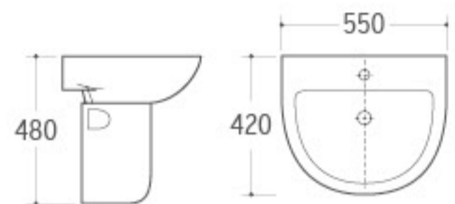
WB-019 Wall-hung Basin Size: 550x420x480mm Wall-hung installation
