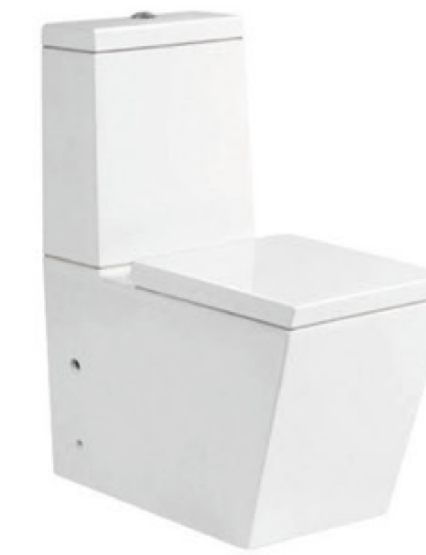
2002 Washdown Two-piece Toilet Size: 660x360x850mm P-trap: 180mm Roughing-in S-trap: 250/300mm Roughing-in
