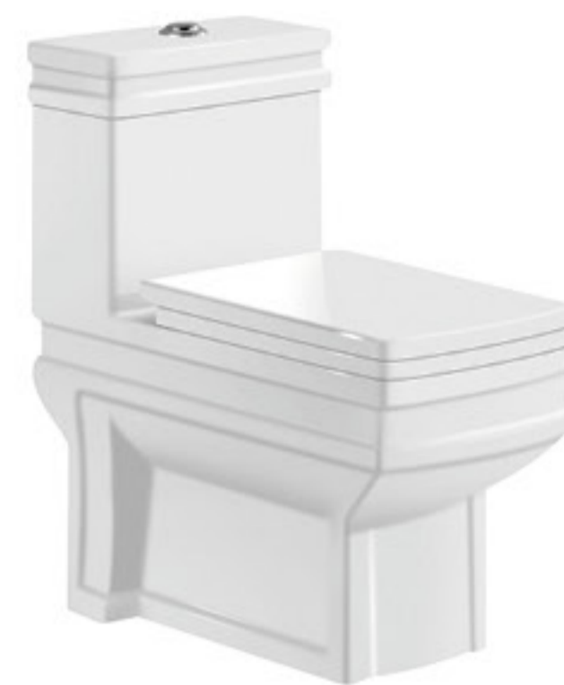
8219 Washdown One-piece Toilet Size: 700x385x760mm P-trap: 180mm Roughing-in S-trap: 250/300mm Roughing-in
