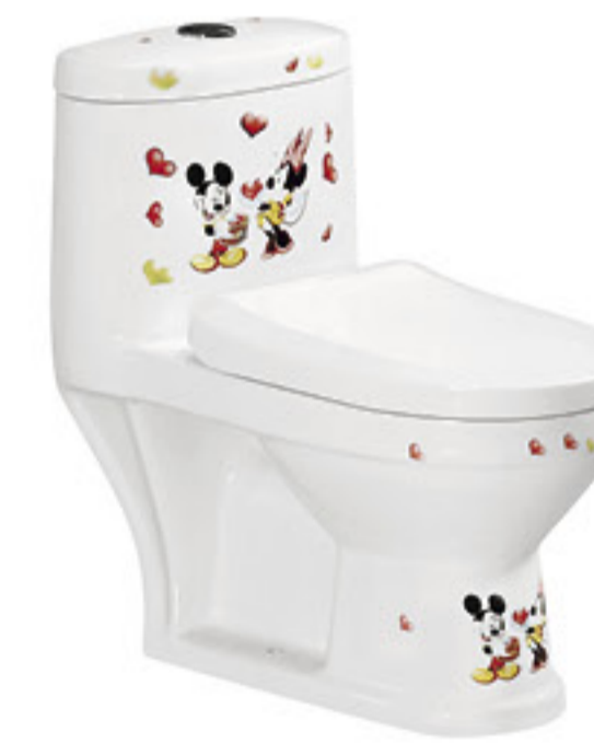
8273F Washdown One-piece Toilet Size: 500x285x530mm P-trap: 120mm Roughing-in S-trap: 200/300mm Roughing-in
