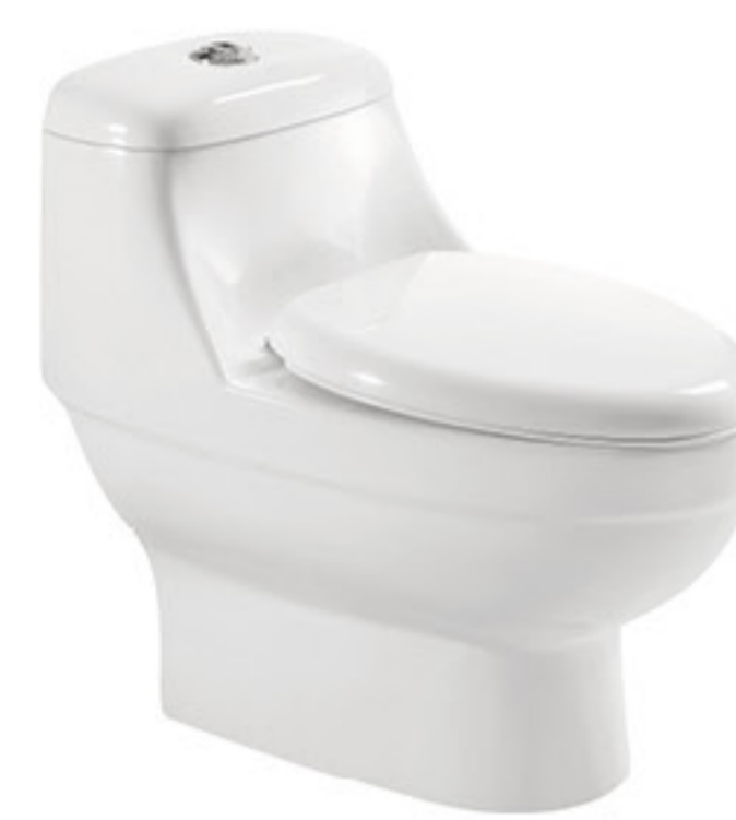
8255B Siphonic One-piece Toilet Size: 730x410x650mm S-trap: 300/400mm Roughing-in
