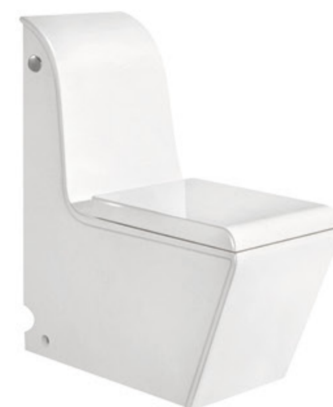
8204 Washdown/Siphonic One-piece Toilet Size: 710x380x820mm P-trap: 180mm Roughing-in S-trap: 250/300mm Roughing-in
