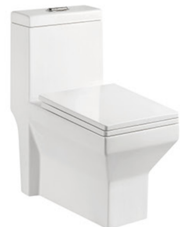
8216 Washdown/Siphonic One-piece Toilet Size: 670x370x760mm P-trap: 180mm Roughing-in S-trap: 250/300/400mm Roughing-in
