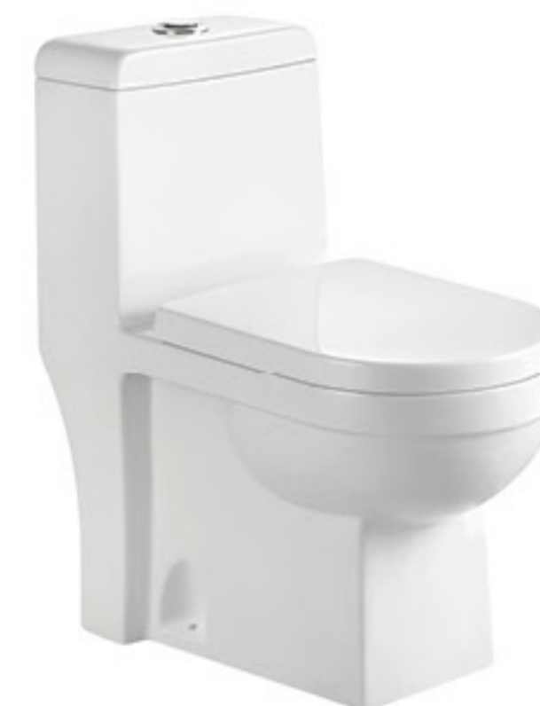
8239 Washdown/Siphonic One-piece Toilet Size: 650x345x730mm P-trap: 180mm Roughing-in S-trap: 250/300mm Roughing-in
