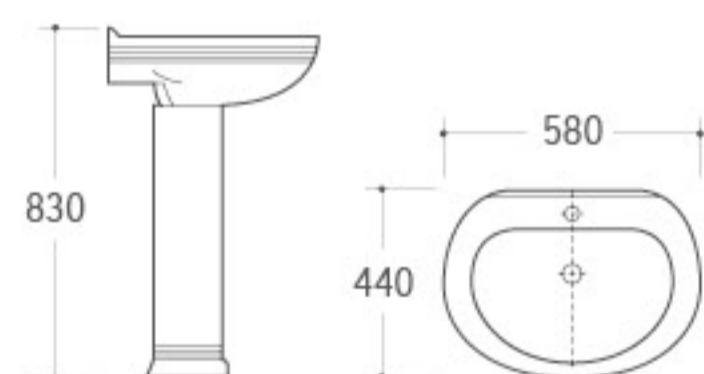
3016 Pedestal Basin Size: 580x440x830mm Fixing to wall with back
