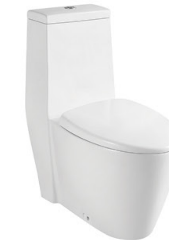
8223 Washdown/Siphonic One-piece Toilet Size: 720x390x835mm P-trap: 180mm Roughing-in S-trap: 250/300mm Roughing-in
