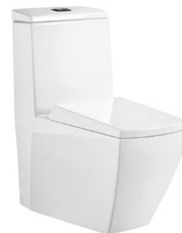
8209 Washdown One-piece Toilet Size: 690x470x785mm P-trap: 180mm Roughing-in S-trap: 250mm Roughing-in
