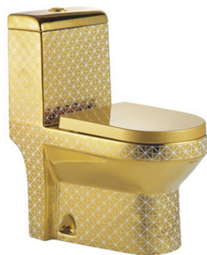
ZJ17104 Washdown/Siphonic One-piece Toilet Size: 690x370x810mm P-trap: 180mm Roughing-in S-trap: 250/300mm Roughing-in
