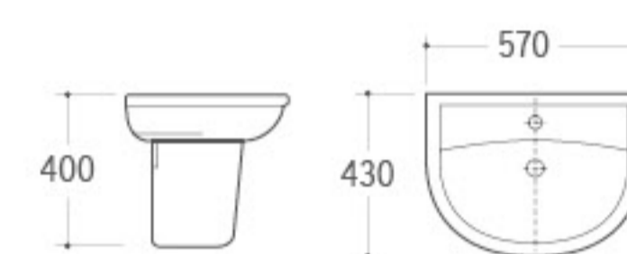
WB-053 Wall-hung Basin Size: 570x430x400mm Wall-hung installation
