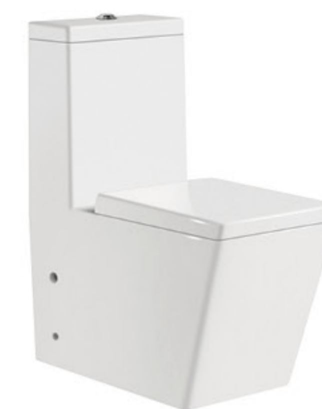
8206 Washdown/Siphonic One-piece Toilet Size: 680x365x840mm P-trap: 180mm Roughing-in S-trap: 250/300mm Roughing-in
