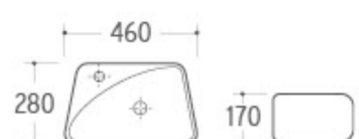
SWB-021 Wall-hung Basin Size: 460x280x170mm Wall-hung installation
