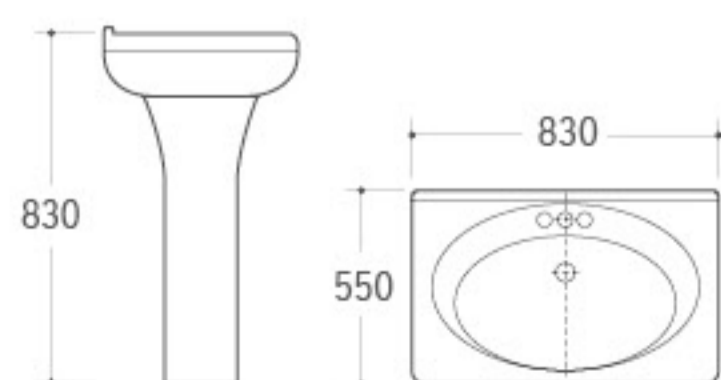
3018 Pedestal Basin Size: 830x550x830mm Fixing to wall with back
