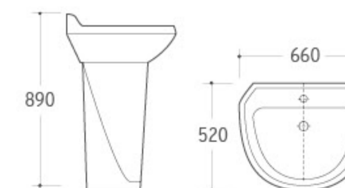
3032P Pedestal Basin Size: 660x520x890mm Fixing to wall with back
