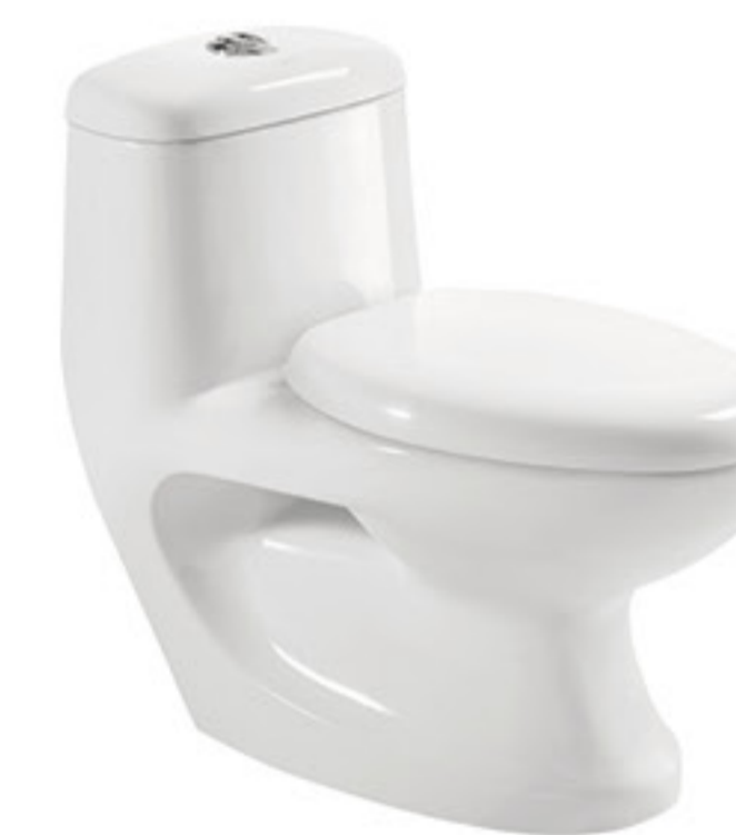
8244 Washdown One-piece Toilet Size: 690x370x640mm P-trap: 180mm Roughing-in S-trap: 250/300mm Roughing-in
