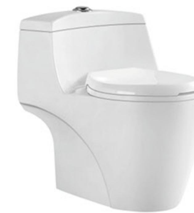
8220 Washdown/Siphonic One-piece Toilet Size: 715x450x650mm P-trap: 180mm Roughing-in S-trap: 250/300mm Roughing-in
