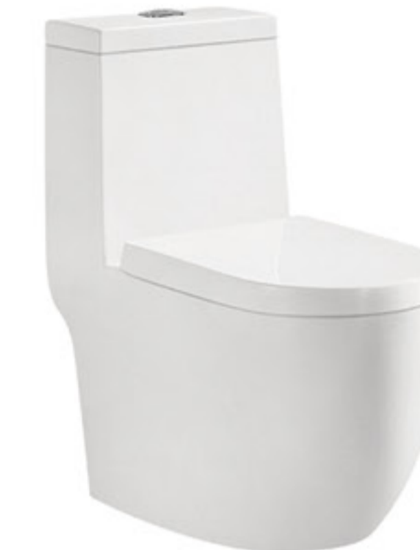
8259 Washdown/Siphonic One-piece Toilet Size: 680x370x780mm P-trap: 180mm Roughing-in S-trap: 250/300/400mm Roughing-in
